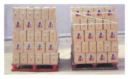
Plastic foil replaced by a band wrapped around the boxes on the upper part of the pile on the
